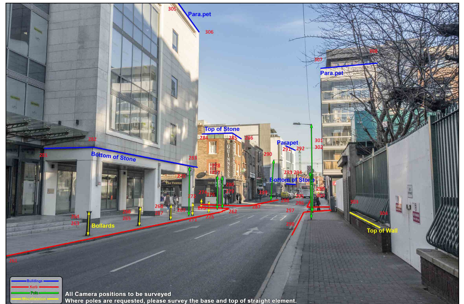
Fig.8: Fixed reference points fully surveyed and numbered.
